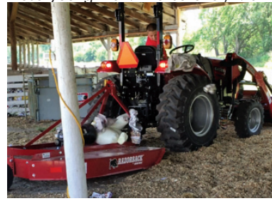
Kyle & Kevin Engel use a stuffed dummy to demonstrate the danger of getting too close to the power take off shaft.
